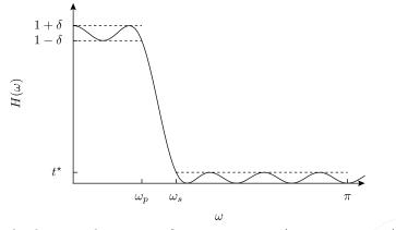
Transfer function for  $n = 10, \delta = 0.05, \omega_p = \pi/4, \omega_s = \omega_p + \pi/8$ .
