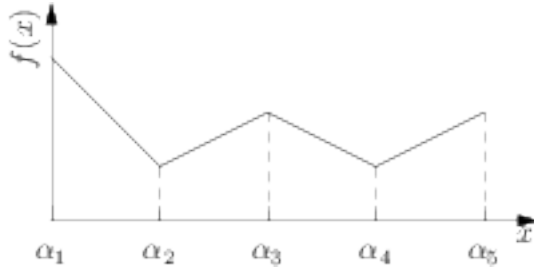
Fig. 6.2: A univariate piecewise-linear non-convex function.
